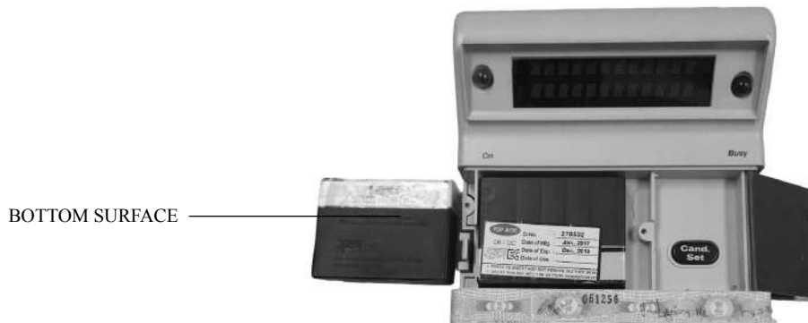
FIG. 20 Installing the Power Pack
